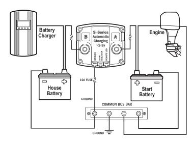
See Wire Size and Fuse Rating charts for connections from Terminals A and B.
