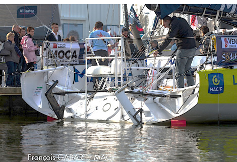
60' IMOCA Macif skippered by François Gabart, Winner of Vendée Globe 2012-2013. Both carbon hydrogenators are mounted on the transom to be immersed and lifted upon request.
