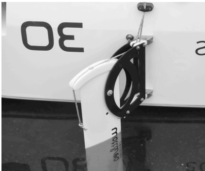
Lifting the hydrogenerator
