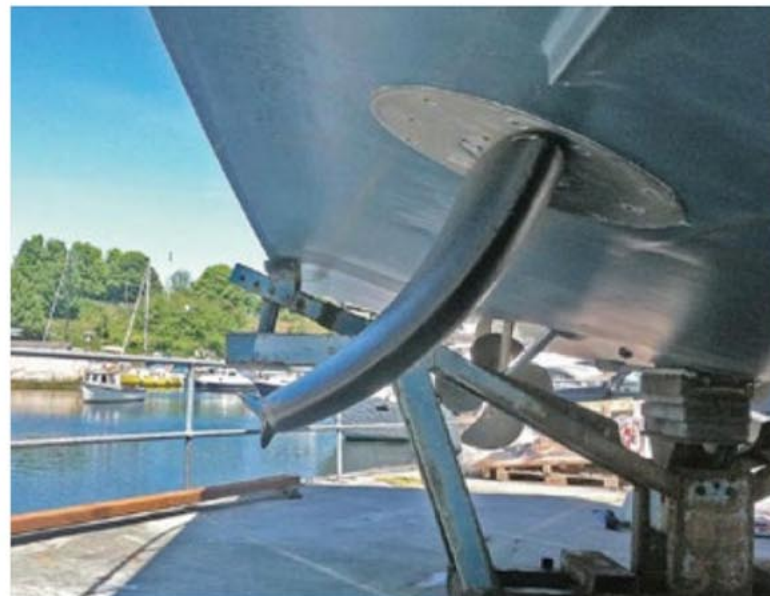
The new curved stabilisers generate more thrust and less drag than straight fins
